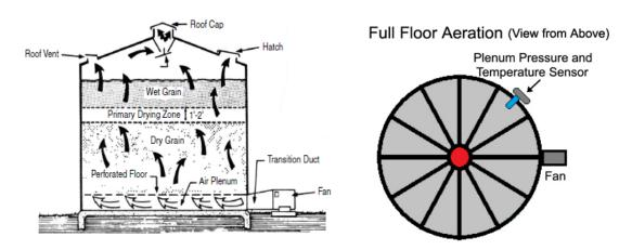
OPI-BVC-REV-08 R-02-08-2017 © 2017 OPIsystems Inc 2. Using a step bit, (shown below) drill a 1 ¼ inch (3.1 cm) hole in the desired location ensuring it is located in the Plenum. (Between the concrete pad and the Aeration floor).
