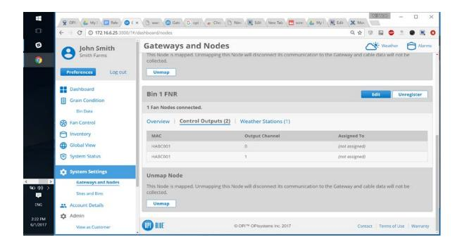
**Note:** The Weather Station Icon will appear at the top right-hand corner once a Fan Node with a Weather Station has been mapped.
