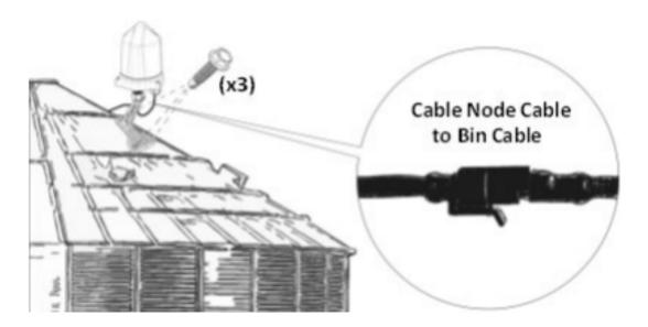
2. Using your Philips screwdriver loosen the three screws located on the outer edge of the base of the Cable Node and open the Cable Node up by lifting the dome off the base.
