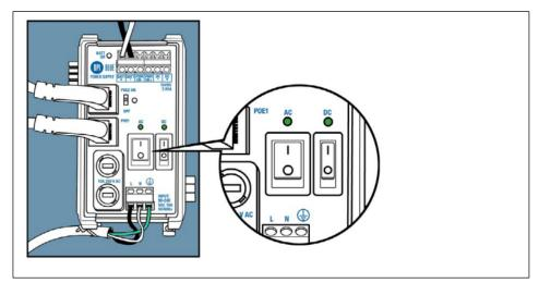
**Note:** When cycling power to the Gateway Node it is important to keep the power switch in the OFF position for 30 seconds before reapplying power. This will ensure the system has completely powered down.
