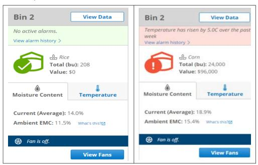
At the bottom of each of the bins that have fan control, the current fan status will be displayed. To drill down further to make changes to the fan status, tap the **View Fans** button to open the **Fan Control** page.
