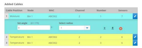
**Note:** When relocating cable(s) you can change the angle in which the cable angle has been set, in addition to changing the radius in which the cable has been positioned.
