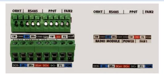
To correctly terminate all connections into the Fan Node, use the **Termination Connection Guideline Chart below.**
