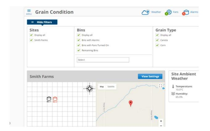
Each bin displayed provides an overview of the current condition of the grain within the structure. If there are moisture and temperature cables in the bin there will be a tab visible for each. The Moisture tab will display the
