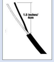
For all wires, use a 20-AWG wire stripper to remove 3/8 inch (1 cm) insulation. This ensures a good consistent termination of all wires. Use a 22-AWG wire stripper for the blue and white communication wires, removing a similar amount of insulation as before.
