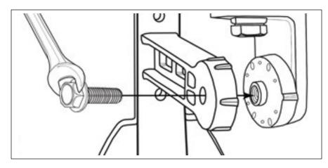
2. Determine the location of the Cable Node on top of the bin roof. Peel the backing off the base of the foot mount and stick into place before bolting down.
