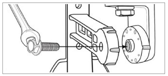
3. Using the cordless drill with the 3/8" Nut Driver, secure the Gateway Node in place with the three self-tapping screws supplied. **Note:** You will need to adjust the position of the Gateway Node on the foot mount in order to attach all three self-tapping screws. Once the screws are in place, use the
