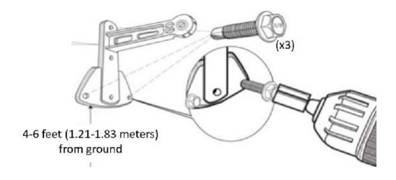
3. Attach the Weather Station to the foot mount using a 7/16-inch wrench and tighten so it is in a vertical position. (Typically, 90 degrees)
