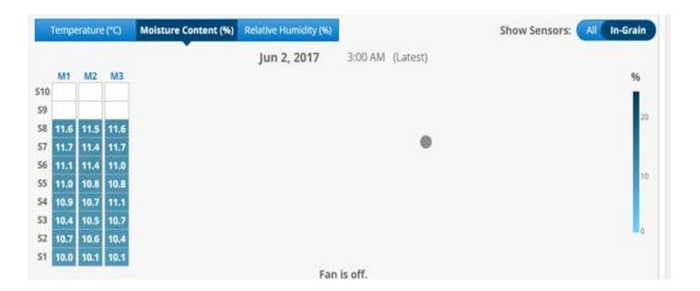
**Note:** By default, the cable data will be displayed for all cable sensors. Using the **Show Sensors** toggle switch the system can be configured to display all sensor data or only the data from the sensors that the system has determined are in the grain.
