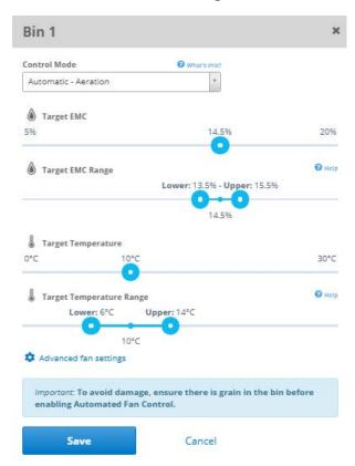
There are also **Advanced Fan Settings** that can be accessed by clicking on the **Advanced Fan Settings** link, located at the bottom of the **Fan Setting Page**. See the Advanced Fan Settings section to get a better understanding of each of these settings and what they mean.
