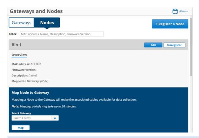
**Note:** If there are multiple Gateways registered use the dropdown list to select the appropriate one the Cable Node needs to be mapped (associated) to.
