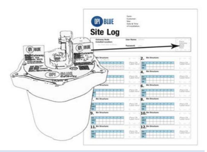
**Note:** When selecting the location for the Gateway Node installation, remember to pick a location that has the best possible line of sight to the bins with the installed Cable Nodes and Fan Node Radios to maximize the communication level between devices. Also, make sure that the Gateway Power Panel Enclosure as access to a 110VAC power outlet.
