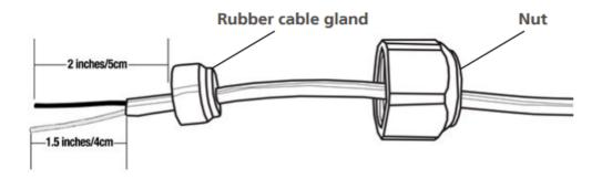
6. Once all the cables have been inserted into each membrane place the gland back inside the strain relief and using the 1 1/16 inch or adjustable wrench reattach it back on the Cable Node base. Repeat this process with the second strain relief if necessary.
