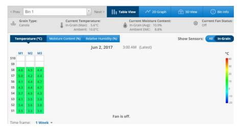
For bins that have moisture cables installed, in addition to being able to view temperature data the humidity data and moisture data are also available to be displayed. For moisture data to appear a Grain Curve must be selected. To add a Grain Curve, go to **System Settings**  $\rightarrow$  **Bins**  $\rightarrow$  (Select Bin) **Grain Info**  $\rightarrow$  **Edit**.
