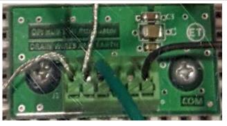
(Left) Black wire terminated in FCOM connection on Fan Node and COM termination on the Attenuator. (Above) Green ground wire and drain wires from Communication Cable (COM2) connected in open left terminations on the Attenuator.
