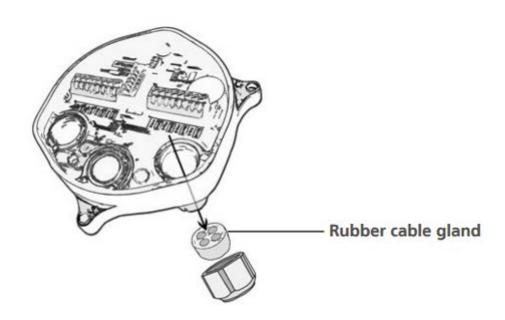
4. Use a small screwdriver to create a tiny opening in the membrane of the gland this way the cable lead wire can be fed through it.
