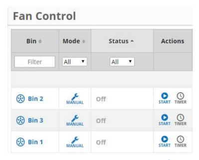
Under the mode column clicking on the MAULICON will cause the **Control Mode** box to appear in which you can select following three options: **Manual**, **Automatic** - **NAD** or **Automatic** - **Aeration**.
