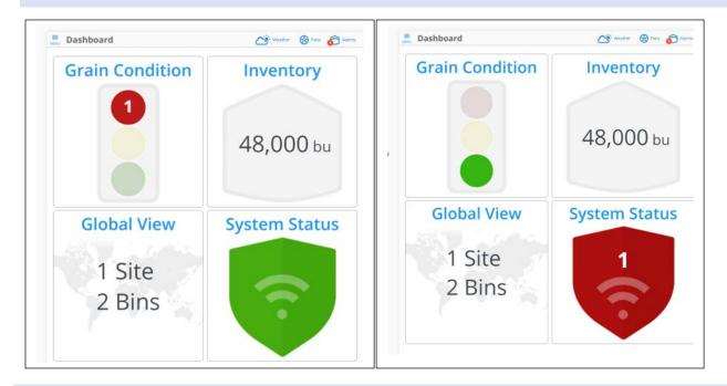
**Note:** Any alarms that are **red** (active/unacknowledged) or **yellow** (active/acknowledged) will be visible on the alarms icon in the top right-hand corner regardless of the screen you are on. Tapping the Alarms Icon will display what the alarm is and provide the options to dismiss or view the alarm. By viewing the alarm condition you will be taken directly to the location of the alarm for viewing.
