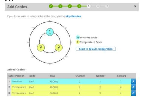
11. \*If necessary you can reposition the cables within the bin to ensure the proper location. Tap the located at the end of a specified cable to start the relocation process.
