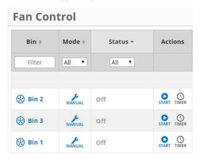
Under the mode column clicking on the MANUAL icon will cause the **Control Mode** box to appear in which you can select following three options: **Manual**, **Automatic** - **NAD** or **Automatic** - **Aeration**.
