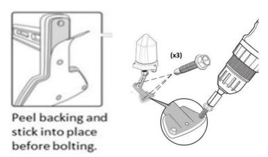
3. Using the cordless drill with the 3/8" Nut Driver, secure the Cable Node in place with the three 3/8" self-tapping screws supplied. **Note:** You will need to adjust the position of the Gateway Node on the foot mount in order to attach all three self-tapping screws. Once the screws are in place, use the 7/16" wrench, tighten the Gateway Node on the foot mount so it is secured in a vertical position.
